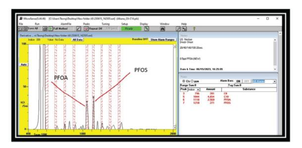
Weight is AEM Membrane: 364mg slice — Heated to 32 degrees C The graphic shows that there is PFOA and PFOS present
