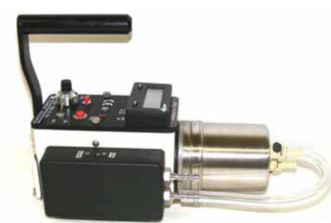
TBM-IC-RN Solid Wall Chamber With Air Pump
