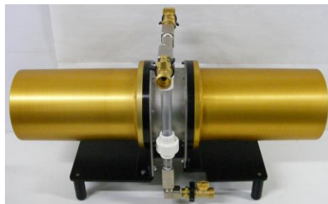
Two Pairs of Matched Photo Multiplier Tubes
